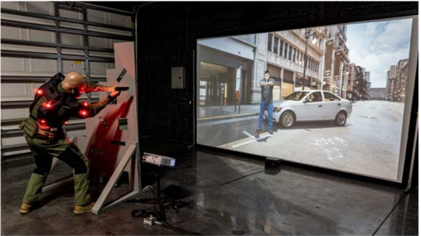
DART Red Fire works with third-party products like the SKIFTECH tactical vest and Scorpion shock band to simulate gun fire from characters within the simulation.
